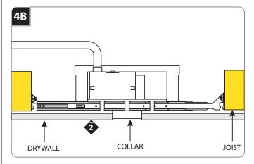
Align the cut out section of drywall with the collar and install the drywall.
