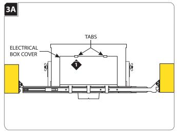
Push up on the tabs on the electrical box and remove the electrical box cover.
