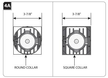
For round trims, mark a 3-7/8" diameter circle on drywall. Cut out the marked section.
