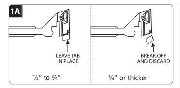
**NOTE:** Skip this section if installing the housing with butterfly brackets.
