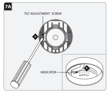
**NOTE:** Lamp housing can tilt 40° vertically. Lines on lamp housing are 5° apart.
