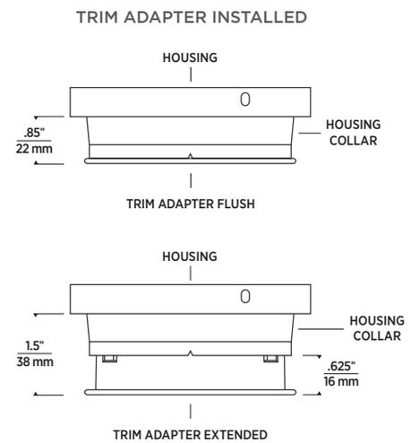
Wood ceiling housings ("WC" designation in the ordering grid) ship with an adjustable trim adapter that inserts into the housing aperture and allows standard ELEMENT 3" flangeless trims to achieve a truly flangeless, flush ceiling appearance in special applications such as wood or stone installation. For use in new construction. Consult installation instructions regarding plenum requirements and ceiling thickness ratios.
