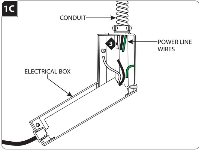
**3** Run the power lines to the desired knockout on the electrical box and fasten the appropriate connector(s) (not included)
