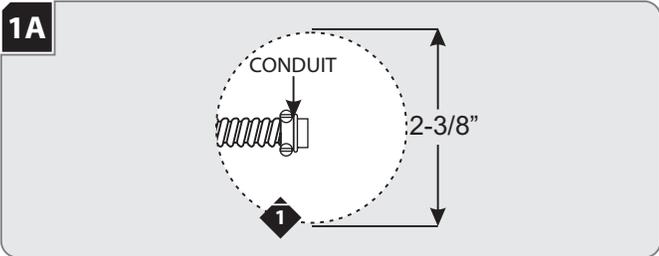
**1** Using a 2-3/8" hole saw, cut a hole into the ceiling at the desired location(s) and route the conduit / power lines to the opening.
