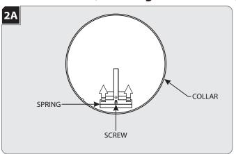
Release the spring by removing the screw.
