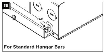
2 If using standard hangar bars bend up and break the bracket tab off with needle nose pliers.
