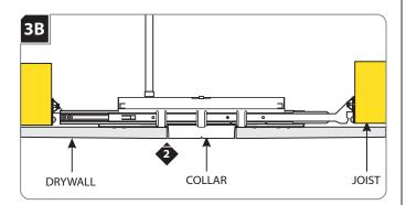
Align the cut out section of drywall with the collar and install the drywall.
