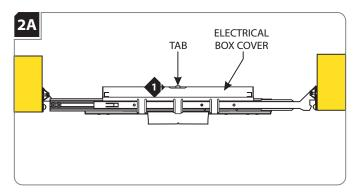
Push up on the tabs on the electrical box and remove the electrical box cover.
