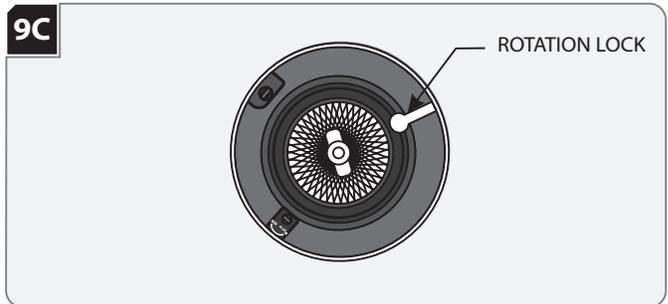
**NOTE:** Lamp housing can rotate 361° horizontally.
