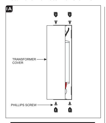
**NOTE:** In order to use small gage wires from the transformer to the electrical box, it is recommended to install the remote transformer near (if possible) the electrical box. See "Low Voltage Wire Size Table" below.
