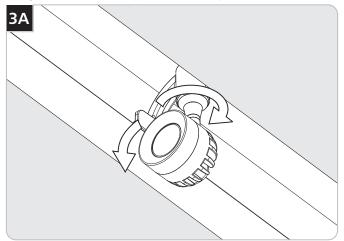
1 Tilt and/or rotate the spot head to the desired location.
