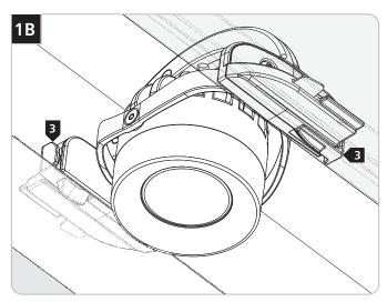
3 Lock the modules into place by rotating locking tabs downward.
