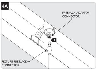
Screw the Fixture FreeJack male connector into the FreeJack female connector.
