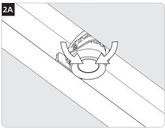
Aim the modules to the desired location by tilting it on either axis.
