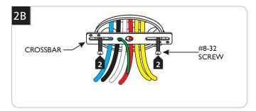
2 Mount the crossbar assembly to the electrical box with the two provided #8-32 screws.
