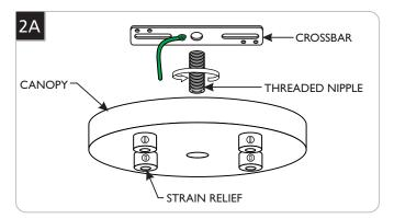
1 Remove the crossbar from the canopy and separate it from the threaded nipple by completely unscrewing it out.
