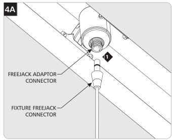
Screw the Fixture FreeJack male connector into the FreeJack female connector.
