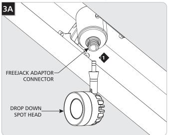
• Screw the drop down spot head into the FreeJack female connector.
