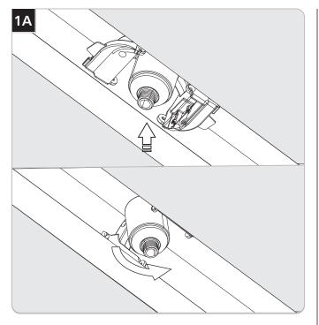
Install the modules into the fixture channel at the desired location and rotate them 90° into place.
