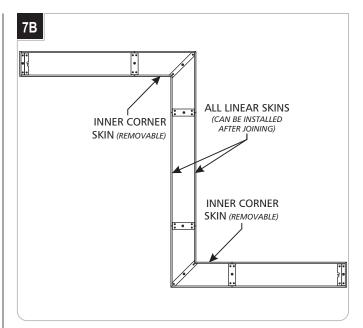
•The inner corner skins can be removed so side skins with outer corner skins on only one end can be installed later.
