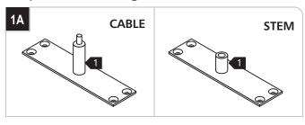
Prepare the hanger plates by mounting the cable grips or stem posts using the screws and lock washers provided.
