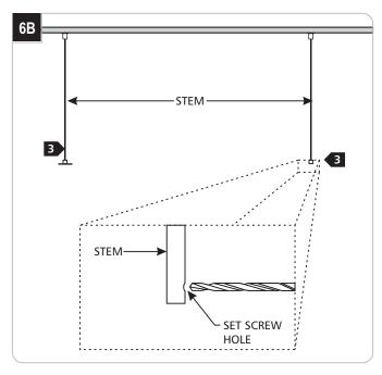
Remove the fixture and drill a hole using a #29 (0.136") drill bit at the marked location in each stem.
