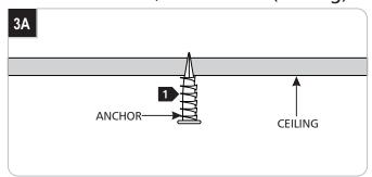
1 At the mark point, tap the anchor into the ceiling up to the threaded portion with a hammer.
