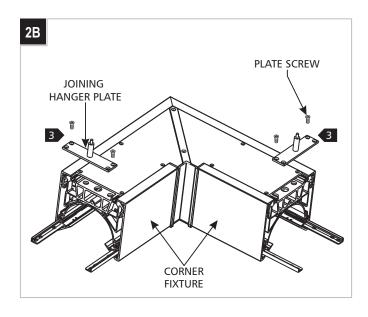
Install two joining hanger plates to the corner fixture using the plate screws without fully tightening them.
