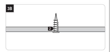
2 Screw the anchor in the rest of the way with a Phillips screwdriver.
