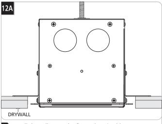
1 Install drywall up to the fixture housing(s).
