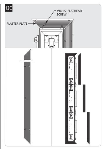
4 Secure the plaster plates to fixture(s) using the supplied #8x1/2 flat head screws:
