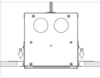
2 If necessary, adjust the fixture height so that the backer flange makes contact to drywall surface.
