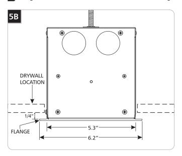
Use the hanger plates to properly support the fixture using threaded rod in accordance with local code. Install the fixture(s) 1/4" lower than the drywall ceiling plane.
