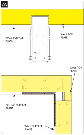
1 To create clearance for the ceiling to wall connector, the wall top plate must be modified, following guidelines in accordance with local building code, to accommodate the fixture's depth.
