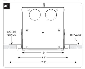
Use the hanger plates to properly support the fixture using the threaded rods in accordance with local code. Install the fixture(s) so that the backer flanges are aligned with the top surface of the drywall.
