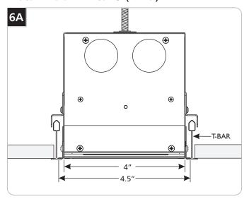
Build a 4.5" on-center grid to accommodate the fixture(s).
