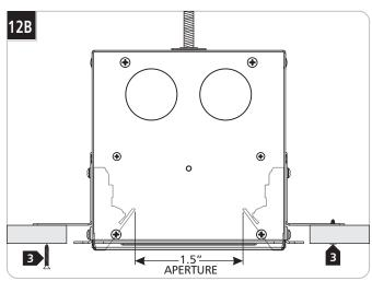
Secure the drywall to the backer flange by either drilling a pilot hole and screwing in sheet metal screws or use self-drilling sheet metal screws.
