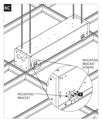
Install two grid mounting brackets to each end of the fixture using the provided bracket screws (8' models require two brackets in the center of the fixture as well).
