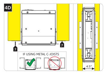
This option uses framing rather than hanger plates to support the fixture. This option is recommended for wall installations and 2" X 4" construction.
