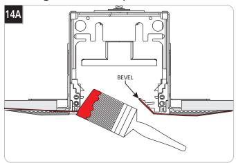
1 The fixture bevel may be painted to match the ceiling color. Take caution not to over paint! This will result in damaging the LEDs.
