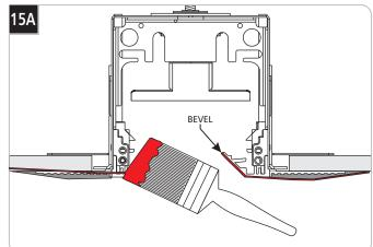
The fixture bevel may be painted to match the ceiling color. Take caution not to over paint! This will result in damaging the LEDs.
