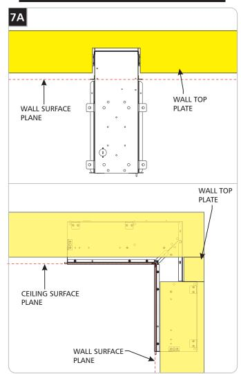
To create clearance for the ceiling to wall connector, the wall top plate must be modified, following guidelines in accordance with local building code, to accommodate the fixture's depth.
