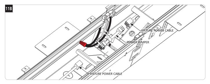
2 Use the power jumpers to connect the fixture power cables together. Keep the jumpers tucked into the notches in the frame so they won't interfere with the installation of the reflectors later.
