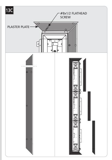
Secure the plaster plates to fixture(s) using the supplied
