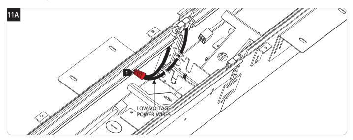
1 Connect the low-voltage power wires together. Pass the wires through the holes in the frame so they won't interfere with the installation of the reflector later.
