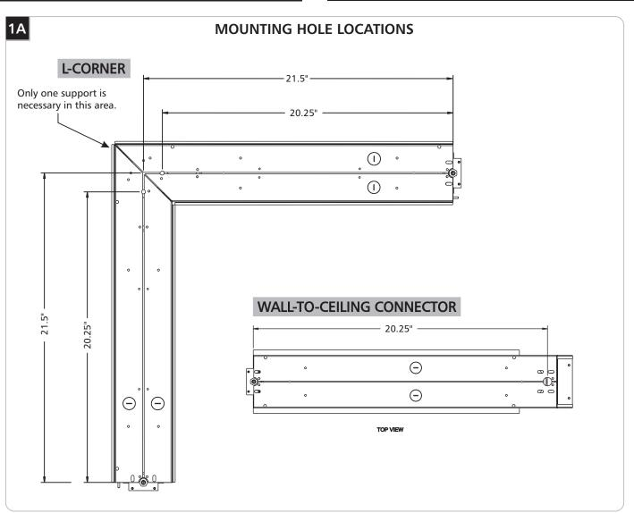
Install threaded rod or tie wire on the centerline of the fixture at the seam between fixtures, at the ends of the run, or using the provided diagrams where necessary. Do not let the threaded rods extend more than 1" into the fixture.
