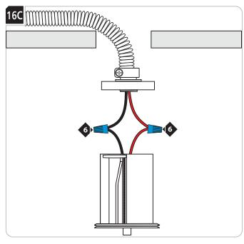
6 Connect the red and black wires in the test switch port to the same color wire in the flexible conduit using wire nuts.
