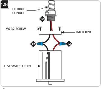
Unscrew the #6-32 screws to open the test switch port.
