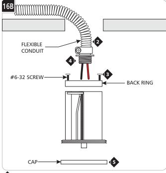
2 Bring the flexible conduit out of the 1-9/16" hole.
