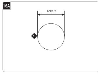
Use a 1-9/16" hole saw to cut out the ceiling or wall where the test switch will be installed.
