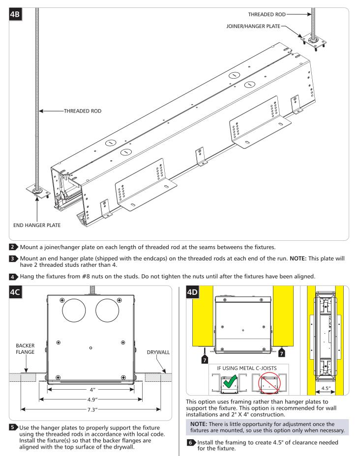
**7** Using wood screws, secure the fixture into the joists by screwing through the backer flanges.
