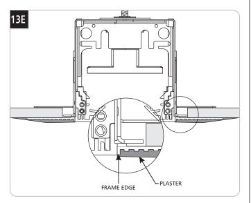
6 Plaster up to the frame edge for a seamless appearance.
