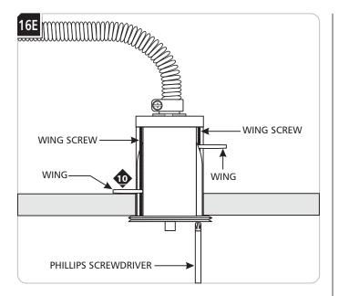
• Tighten the two phillips screws (an electric screwdriver will help) until the wings secure the test switch port into the hole.
