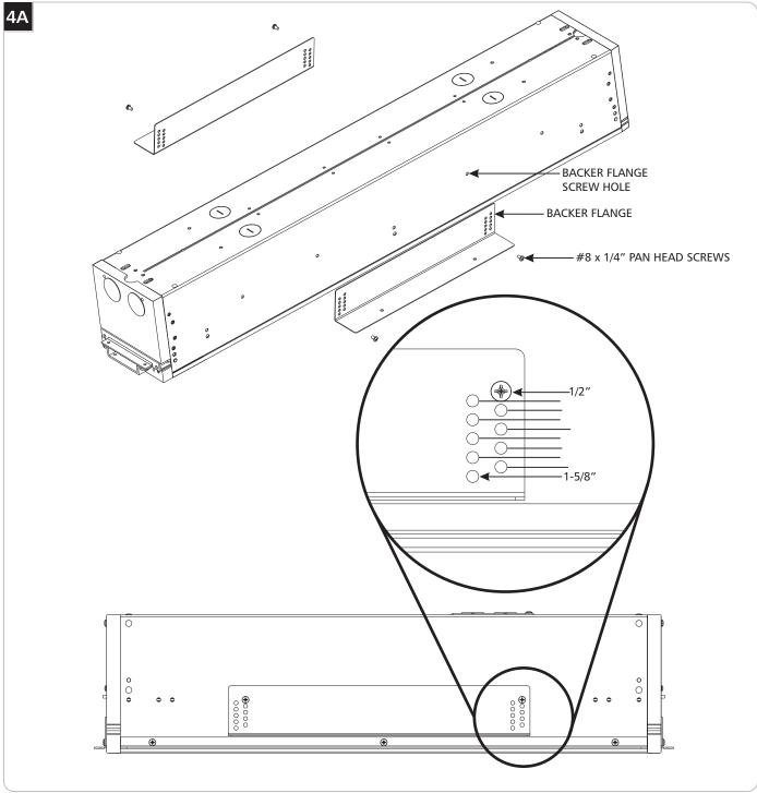
Set the height of the backer flange according to the finished ceiling thickness (maximum 1-5/8" ceiling thickness): install the flange at the appropriate height using the #8 x 1/4" pan head screws. The holes are spaced 1/8" apart.
