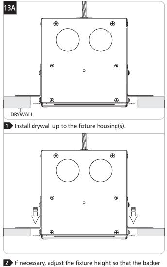
flange makes contact to drywall surface.
