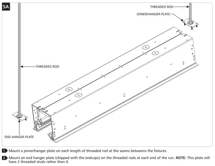
B Hang the fixtures from #8 nuts on the studs. Do not tighten the nuts until after the fixtures have been aligned.
