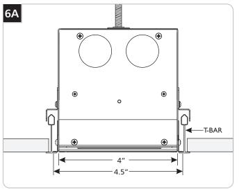
Build a 4.5" on-center grid to accommodate the fixture(s).
