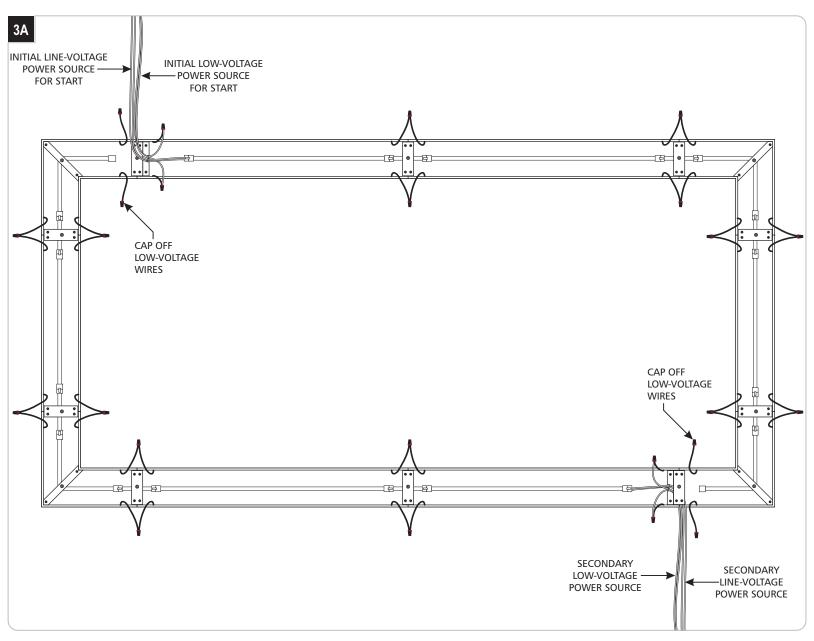
For an enclosed run, if the total run length is more than 80', multiple line-voltage power supplies must be used.
