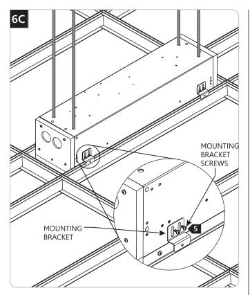
Install two grid mounting brackets to each end of the fixture using the provided bracket screws (8' models require two brackets in the center of the fixture as well).
