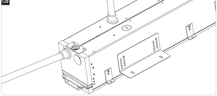
Install the conduit to the knock-outs provided in the endcaps or along the body of the fixture itself.
