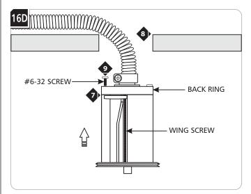
**7** Replace the back ring onto the test switch port so the end of the wing screws are properly placed in the two blind holes.
