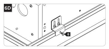
6 To further secure the fixture or per local code, use the screws slots on the sides of the brackets to secure the fixture to the T-bar.
