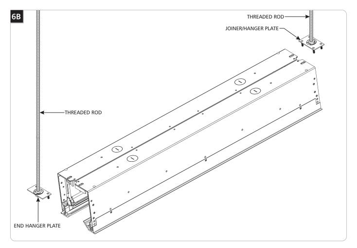
2 Mount a joiner/hanger plate on each length of threaded rod at the seams betweens the fixtures.
