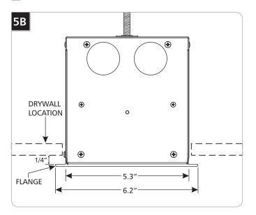
Use the hanger plates to properly support the fixture using threaded rod in accordance with local code. Install the fixture(s) 1/4" lower than the drywall ceiling plane.
