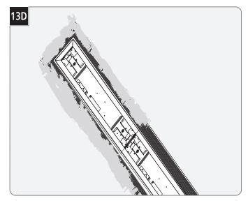
**5** Properly plaster onto the plaster flange and drywall.
