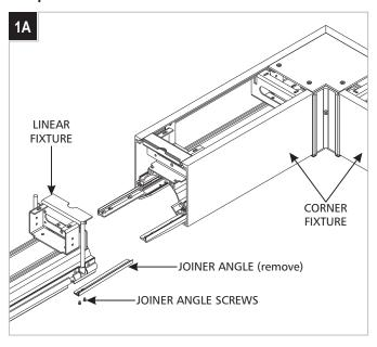
The preparation of the linear fixtures is described in the installation instructions included with them. One additional preparation step is necessary when using a corner fixture:
