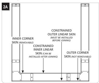
The previous instructions suggest connecting the units together with the side skins removed for ease of access. If installing 2 or more corners in a run, where linear units will be constrained at both ends by corners, please note the following:
