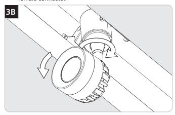
2 Tilt and/or rotate the spot head to the desired location.
