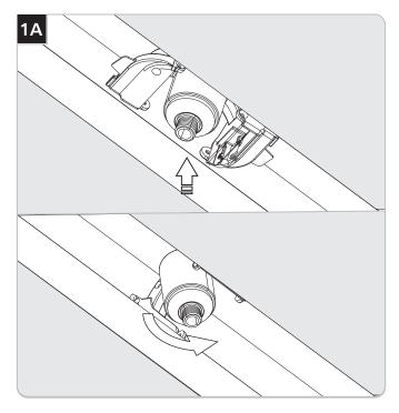
Install the modules into the fixture channel at the desired location and rotate them 90° into place.
