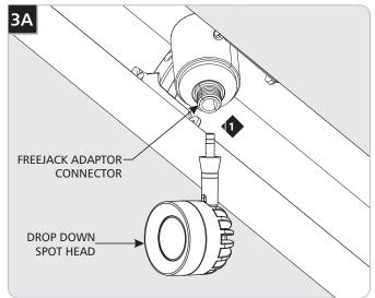
Screw the drop down spot head into the FreeJack female connector.
