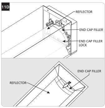
Unlock the end cap filler and ensure that it is flush with the reflector.
