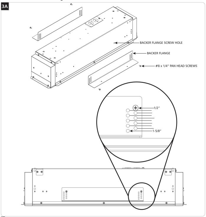
1 Set the height of the backer flange according to the finished ceiling thickness (maximum 1-5/8" ceiling thickness): install the flange at the appropriate height using the #8 x 1/4" pan head screws. The holes are spaced 1/8" apart.
