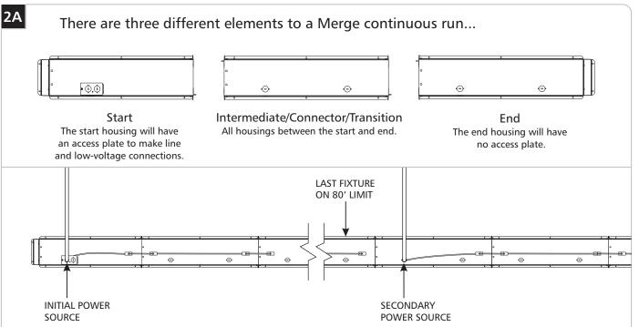
The line-voltage section of the fixture run will be powered at the start of the run, then interconnected with jumper cables to a maximum of 80'. For a longer run, sections may be isolated by simply not using a jumper. The secondary power source must be spliced to the wiring harness and connected to the fixture using one of the provided knockout locations.
