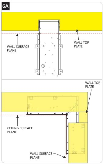
1 To create clearance for the ceiling to wall connector, the wall top plate must be modified, following guidelines in accordance with local building code, to accommodate the fixture's depth. Use section 3 to install the wall to ceiling connector.
