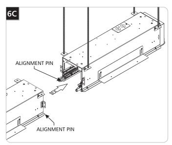
4 Using the alignment pins as a guide, slide the next fixture against the already installed fixture and secure the fixture in place using the preferred mounting method.
