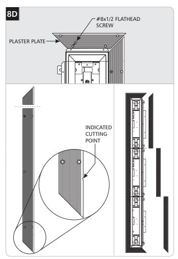
Secure the plaster plates to fixture(s) using the supplied #8x1/2 flat head screws:
