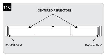
Slide the reflector(s) towards the center of the fixture/run so that there are equal gaps on each end.
