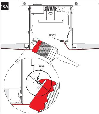
1 The fixture bevel may be painted to match the ceiling color. Take caution not to over paint! This will result in damaging the LEDs.
