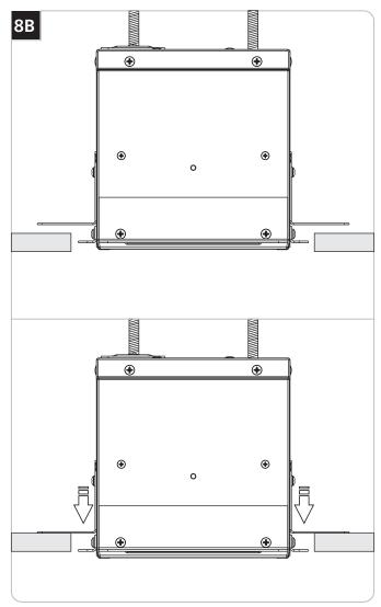
2 If necessary, adjust the fixtures height so that the backer flange makes contact to drywall surface .
