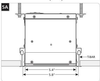
Build a 6" on center grid to accommodate the fixture(s)(see next diagram).
