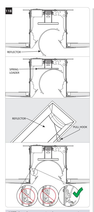
**NOTE:** If your fixture run consists of corner connectors, the corner reflectors should be installed prior to the linear reflectors.
