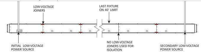
The low-voltage section of the fixture run will also be powered at the start of the run, then interconnected with low-voltage joiners to a maximum of 40'. Sections of the run may be isolated by simply not installing the low-voltage joiners and the run may be powered by multiple transformers at different ends to power longer runs.
