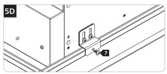
To further secure the fixture or per local code, use the screws slots on the sides of the brackets to secure the fixture to the T-bar.
