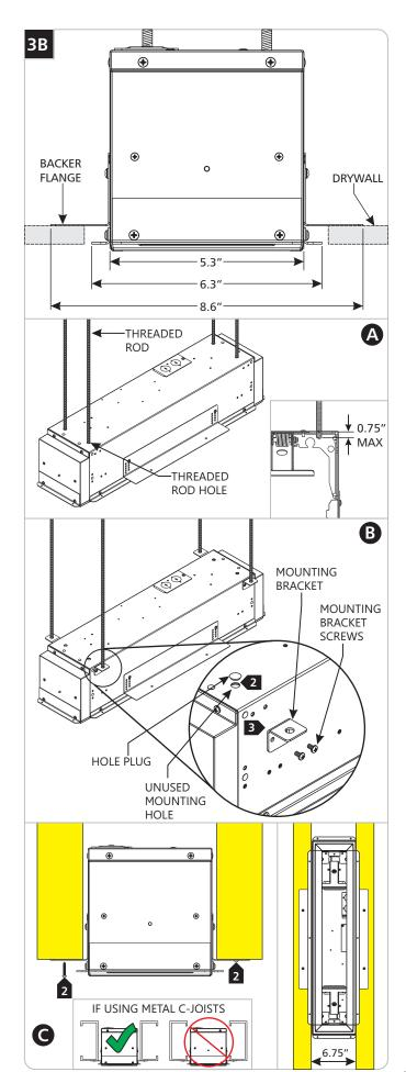
Install the fixture(s) so that the backer flange is aligned with the drywall plane using one of the following options. If installing a continuous run, see section 6 for assembly details once an installation method has been determined:
