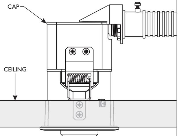
**NOTE:** ENNCONCP is required only when low-voltage wires are being routed through metal conduit and an MC connector is used at the fixture. Access above the ceiling/installation surface is required to use ENNCONCP.
