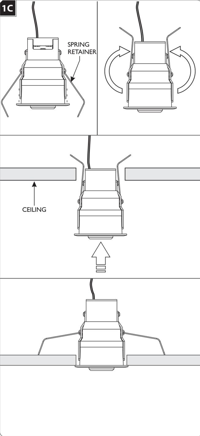
**7** Rotate the spring retainers completely up and insert the fixture into ceiling until it is securely in place.
