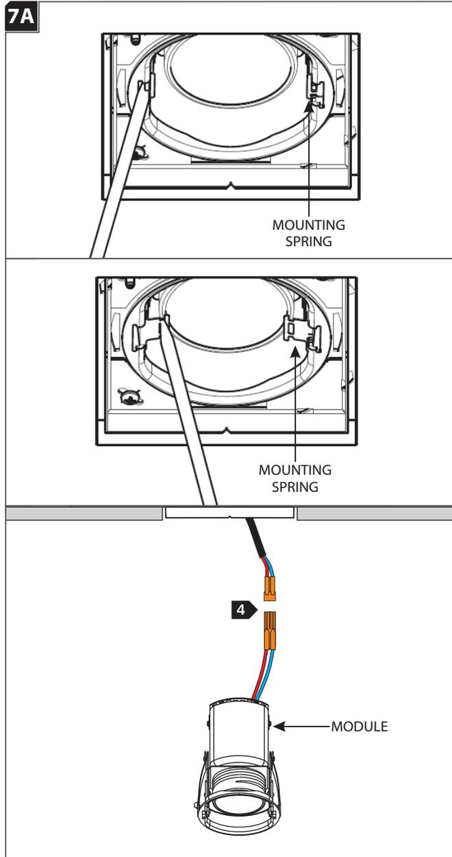
**Note:** The module must be removed in order to access the junction box or replace the optic.
