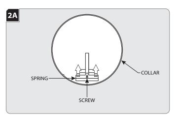
Release the spring by removing the screw.
