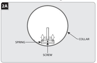
Release the spring by removing the screw.
