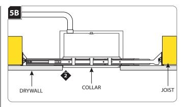
Align the cut out section of drywall with the collar and install drywall.
