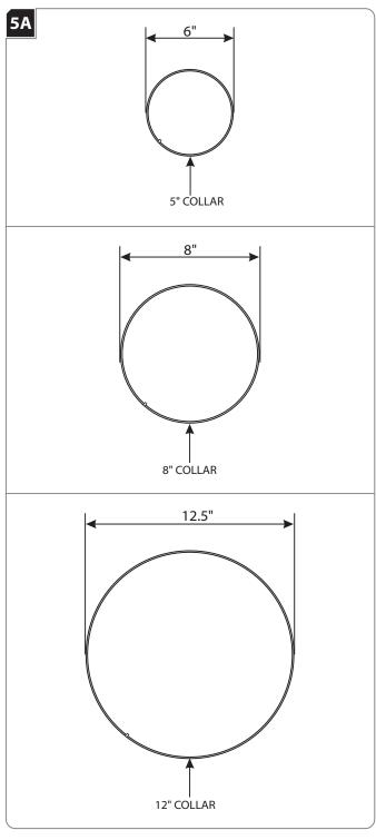
Depending on the fixture's collar size, mark an appropriate sized diameter circle on drywall. Cut out the marked section.
