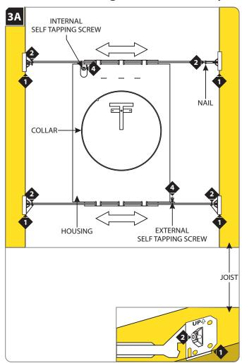
**NOTE:** The adjustable bars can be mounted to joists that are spaced 16" - 24" apart.
