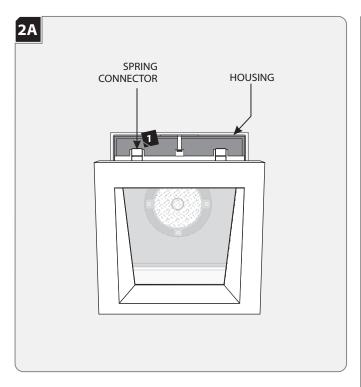
Align the trim spring connectors with the inner edge of the housing.
