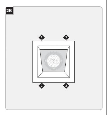
Gently push the trim into the housing so that the four spring connectors snap into place.
