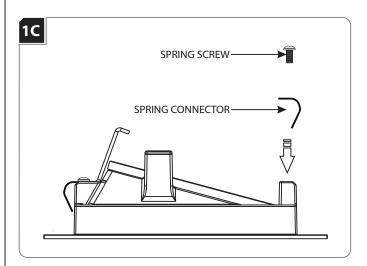
Install the small spring connectors and secure them by reinstalling the spring screws.
