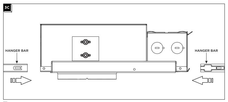
3 Slide the hangar bars into the bracket.
