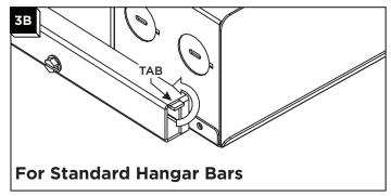
If using standard hangar bars bend up and break the bracket tab off with needle nose pliers.
