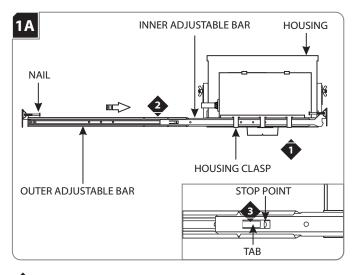
Slide the inner adjustable bar completely through the three housing clasps. Make sure the nail is on top.
