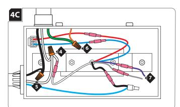
Connect the neutral power line wire to the white transformer wire with a wire nut.
