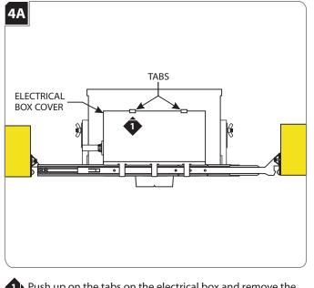
• Push up on the tabs on the electrical box and remove the electrical box cover.
