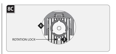
**NOTE:** Lamp housing can rotate 361° horizontally.
