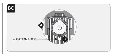
**NOTE:** Lamp housing can rotate 361° horizontally.
