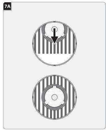
Ensure that the lens assembly is centered to the aperture by pulling the assembly to the center of the housing. When centered the locking pin will be engaged.
