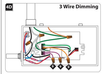
For 3 wire driver applications, properly connect the orange (dimmed hot) and the two purple wires (dimming/digital bus).
