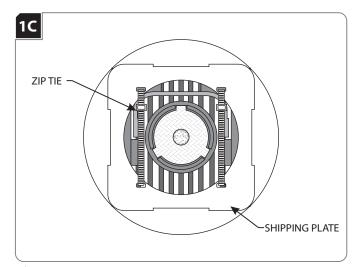
6 Carefully cut and remove the zip ties to remove the shipping plate.
