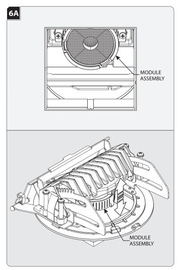
To adjust the height, grip the module assembly and push up to minimize glare and flash on the trim. Pull down on the module assembly for maximum light output and efficiency.
