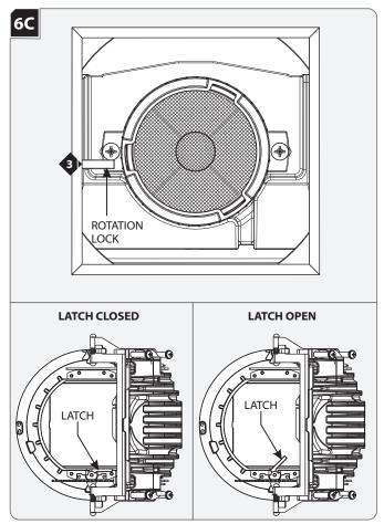
**NOTE:** Lamp housing can rotate 361° horizontally.
