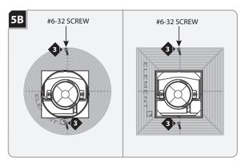
Secure the plaster ring in place with the two provided flat head #6-32 screws. Make sure that the screws penetrate through the drywall into the housing screw holes.
