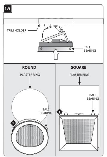
Align the trim ball bearings with the inner edge of the plaster ring. Make sure the lamp and trim are pointed in the same direction. There are printed markings on the trim that indicate "TO LIGHTED WALL."
