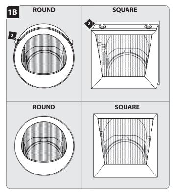
Push the trim into the plaster ring so that the ball bearings snap into the plaster ring walls.
