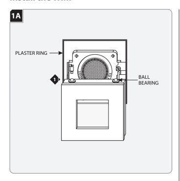
Align the trim ball bearings with the inner edge of the plaster ring.
