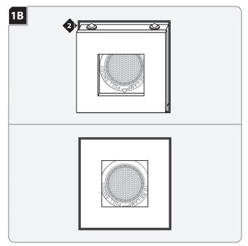
Push the trim into the plaster ring so that the four ball bearings snap into the plaster ring walls.
