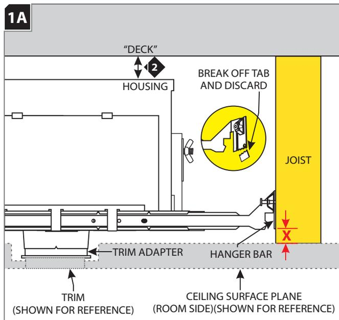
For a ceiling thickness between 3/8" and 1-1/2", use the provided dimensions or equation to determine the distance (X dimension) between the bottom of the hanger bar and the bottom of the joist.
