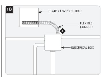
Attach flexible conduit (not included) to an electrical box and feed the conduit out of the cutout.
