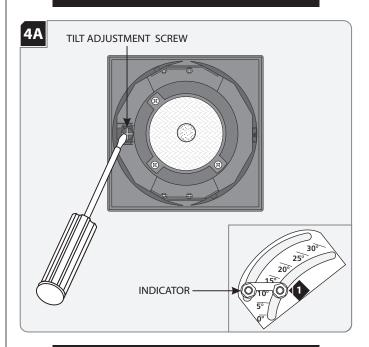
**NOTE:** Lamp housing can tilt 30° vertically. Lines on lamp housing are 5° apart.
