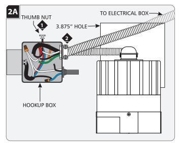
1 Loosen the thumbnut and remove the cover from the hookup box.
