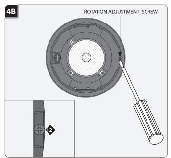
**NOTE:** Lamp housing can rotate approximately 180° horizontally.
