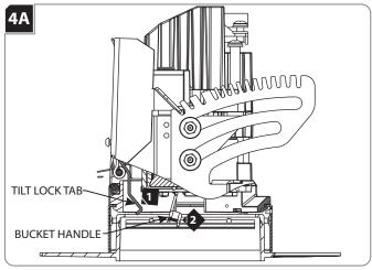
To unlock tilt, pull tilt lock tab towards optic.
