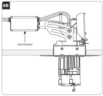
4 Pull the heatsink, module and driver through the aperture.
