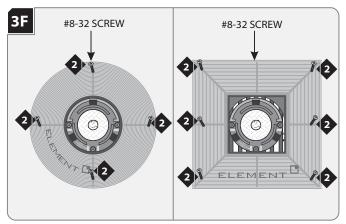
Secure the plaster ring in place by screwing the four provided flat head #8-32 screws into the four previously placed drywall anchors.
