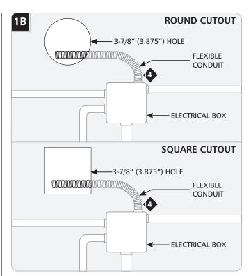
Attach flexible conduit (not included) to an electrical box and feed the conduit out of the hole.
