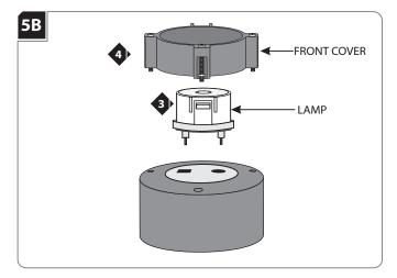
Use **ONLY 18 WATT** proprietary Element Lighting LED lamp.
