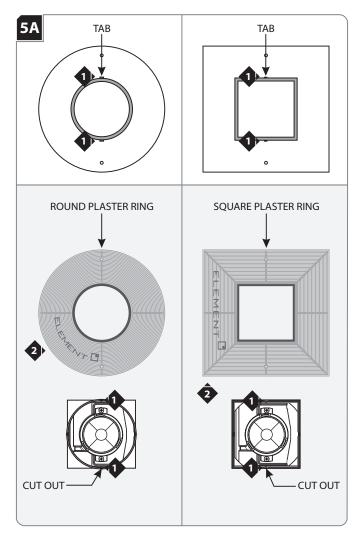
Line up the two tabs in back of the plaster ring with the two cut out sections of the collar's inside edge.
