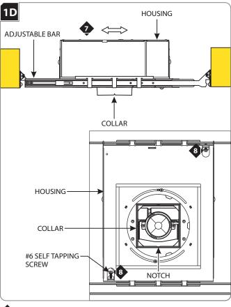
Adjust the collar position (horizontal position) by sliding the housing on adjustable bars.
