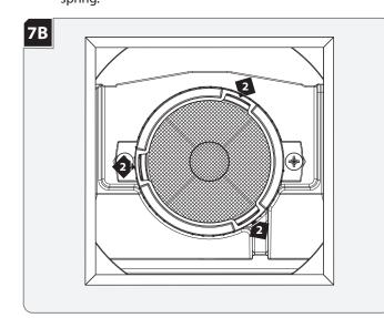
Line up tabs of the lens holder spring with the notches on the optic holder and push the lens holder spring on.
