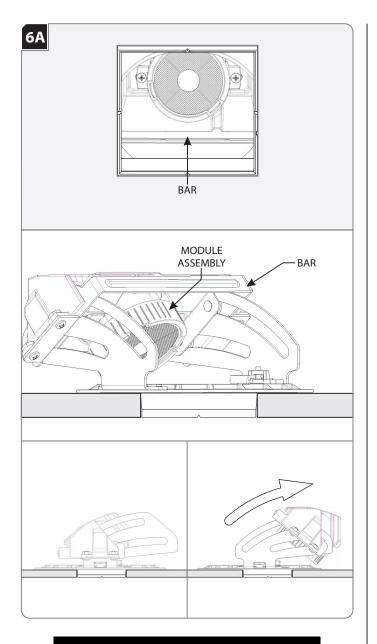
**NOTE:** Lamp housing can tilt 40° vertically. Lock intervals are 2.5° apart.
