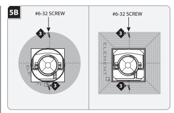
3 Secure the plaster ring in place with the two provided flat head #6-32 screws. Make sure that the screws penetrate through the drywall into the housing screw holes.
