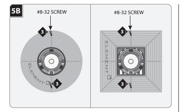
Secure the plaster ring in place with the two provided flat head #8-32 screws. Make sure that the screws penetrate through the drywall into the housing screw holes.
