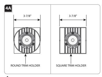
**1** For round trims, mark a 3-7/8" diameter circle on drywall. Cut out the marked section. For square trims, mark a 3-7/8" square on drywall. Cut out
