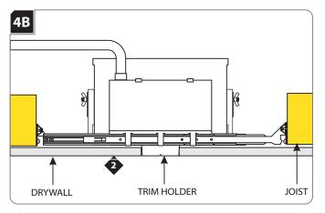
2 Align the cut out section of drywall with the trim holder and install drywall.
