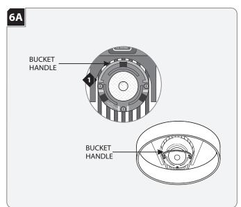
To adjust the height, push up the lamp cartridge assembly to minimize glare and flash on the trim. Pull down the assembly using the bucket handle for maximum light output and efficiency.
