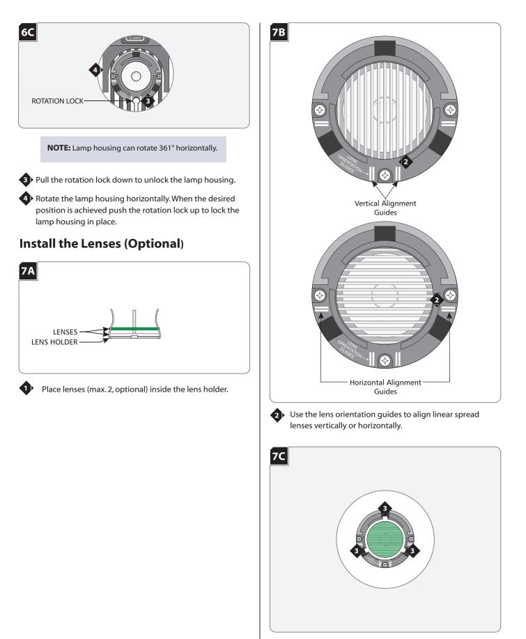
Line up the legs of the lens holder with the notches on the lamp holder and push the lens holder on.
