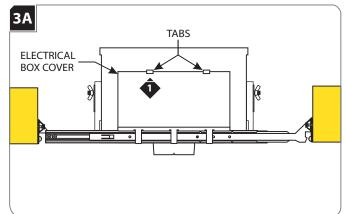
Push up on the tabs on the electrical box and remove the electrical box cover.
