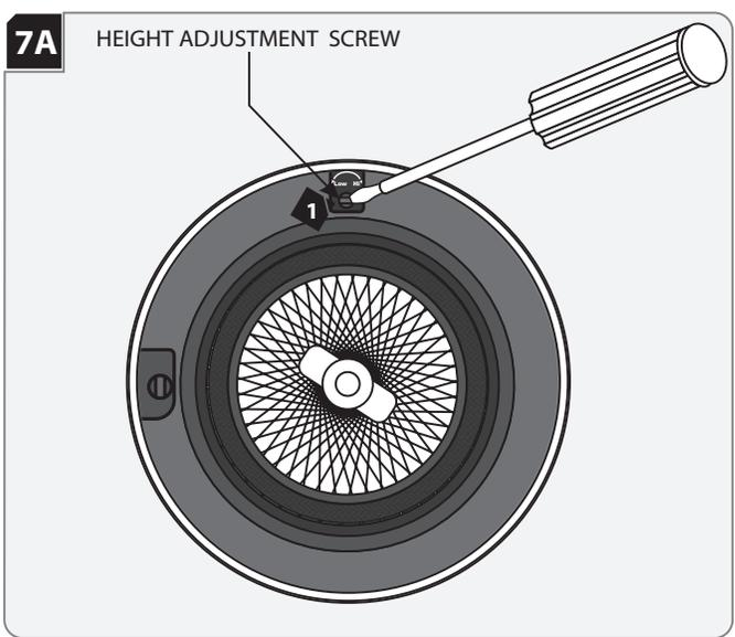
1 To adjust the height rotate the height adjustment screw. Adjust upward to minimize glare and flash on the trim or downward for maximum light output and efficiency.
