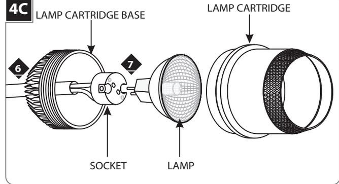
Use **MAX 50 Watt** Type MR16 Halogen Lamp.
