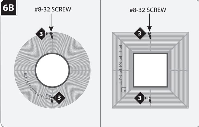
3 Secure the plaster ring in place with the two provided flat head #8-32 screws. Make sure that the screws penetrate through the drywall into the housing screw holes.
