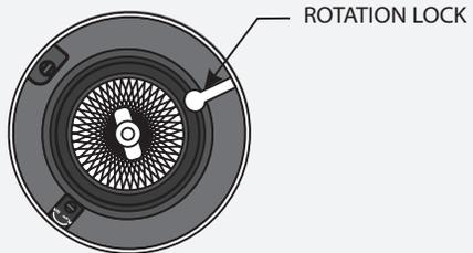
**NOTE:** Lamp housing can rotate 361° horizontally.
