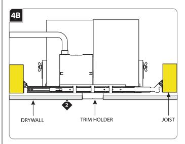
Align the cut out section of drywall with the trim holder and install the drywall.
