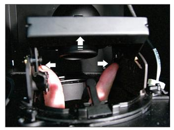
4 Squeeze the tabs to release the lamp housing and push the housing back.
