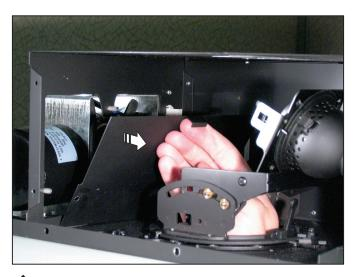
6 Pull the handle on the access door and remove the door.
