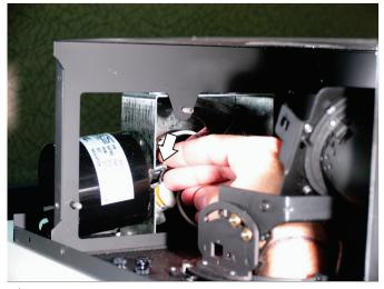
Remove the large wing nut inside the electrical box. This wing nut holds the transformer in place.
