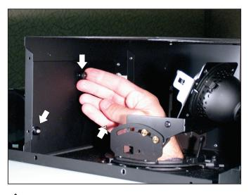
5 Remove the three thumb nuts on the access door.
