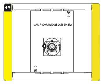
• Pull the snoot to remove the lamp cartridge assembly.
