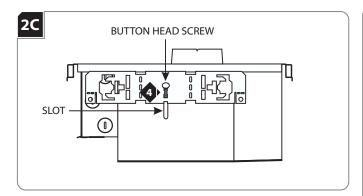
Place the button head screw through the square cut out of the butterfly bracket into the housing slot.
