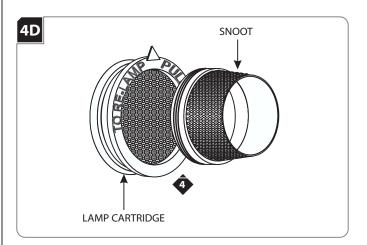
Replace and tighten the snoot completely to the lamp cartridge.
