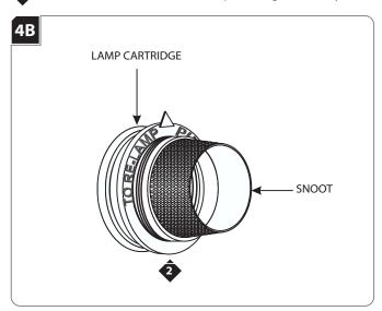
Unscrew the snoot from the lamp cartridge.
