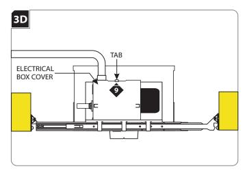
Replace the electrical box cover. Make sure that the top edge of the cover snaps under the tab.
