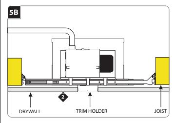
Align the cut out section of drywall with the trim holder and install drywall.
