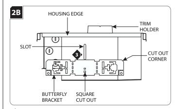
Line up the square cut out section of the butterfly bracket with the housing slot. Make sure the cut out corner of the butterfly bracket is against the housing edge.
