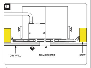
2 Align the cut out section of drywall with the trim holder and install the drywall.
