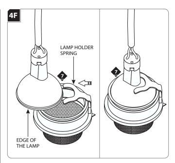
**7** Slide the lamp holder spring completely onto back of the MR16 lamp so that the edge of the lamp snaps into the lamp cartridge assembly.
