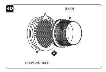
4 Replace and tighten the snoot completely to the lamp cartridge.
