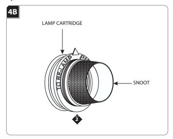
2 Unscrew the snoot from the lamp cartridge.
