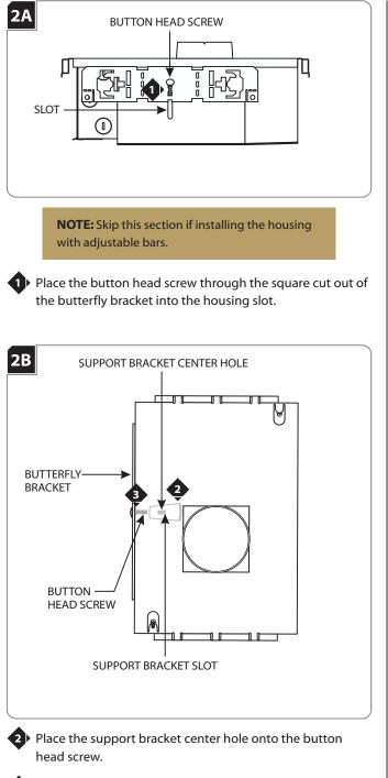
3 Push the support bracket slots against the butterfly bracket tabs.
