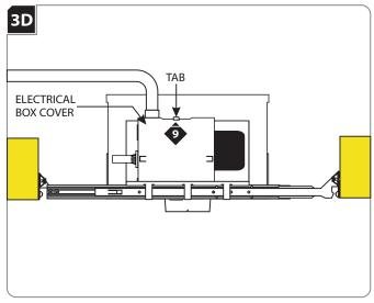
PREPLACE the electrical box cover. Make sure that the top edge of the cover snaps under the tab.
