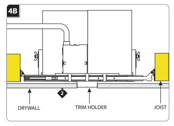
Align the cut out section of drywall with the trim holder and install the drywall.
