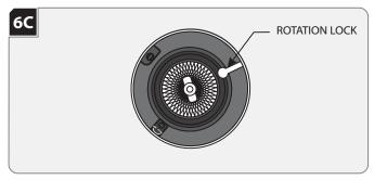
**NOTE:** Lamp housing can rotate 361° horizontally.
