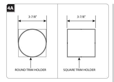
For round trims, mark a 3-7/8" diameter circle on drywall. Cut out the marked section.
