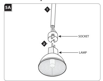
Use **MAX 50** Watt Type MR16 Halogen Lamp.
