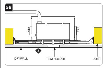
Align the cut out section of drywall with the trim holder and install drywall.
